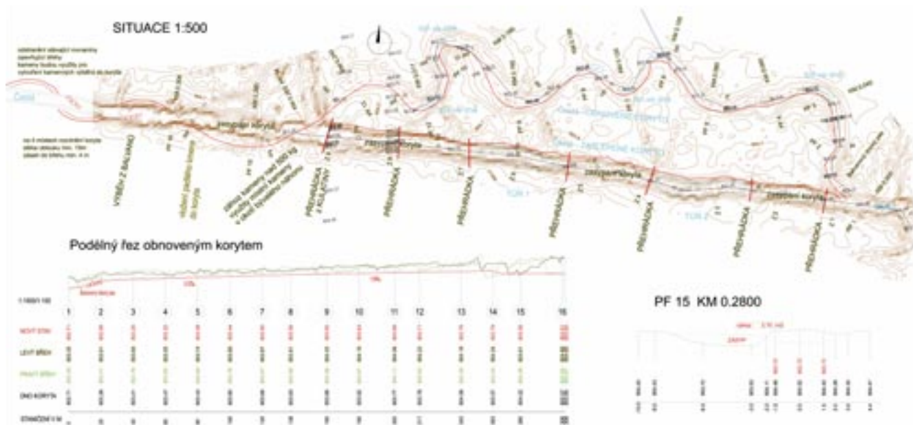
Fig. 130: Situation drawing, longitudinal and cross-section of the newly shaped bed of the Častá river from the technical documentation elaborated for restoration of the Stráženská slat' site, prepared by Martin Dobeš, January 2022
