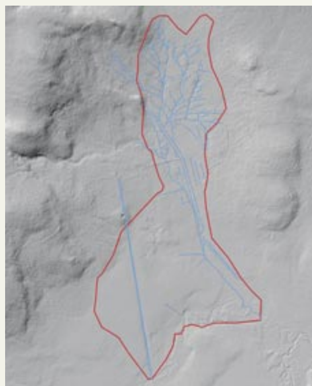
Fig. 241: Scheme of the drainage based on LIDAR images, Nové Údolí
