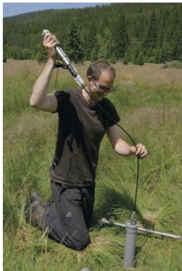
Fig. 183: Pressure sensor for measuring water table TSH22-1-2 (left) and insertion of the sensor connected to the datalogger into a plastic borehole used in Šumava (right), June 2019 (I. Buřková)
