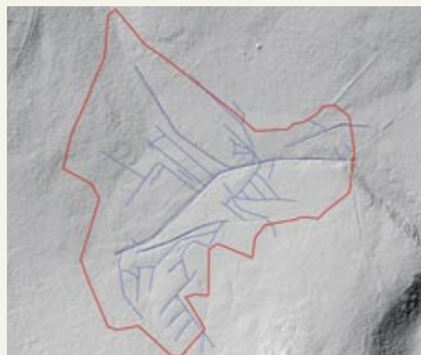
Fig. 218: Scheme of the drainage system at the Vchynice-Tetov site based on LIDAR images
