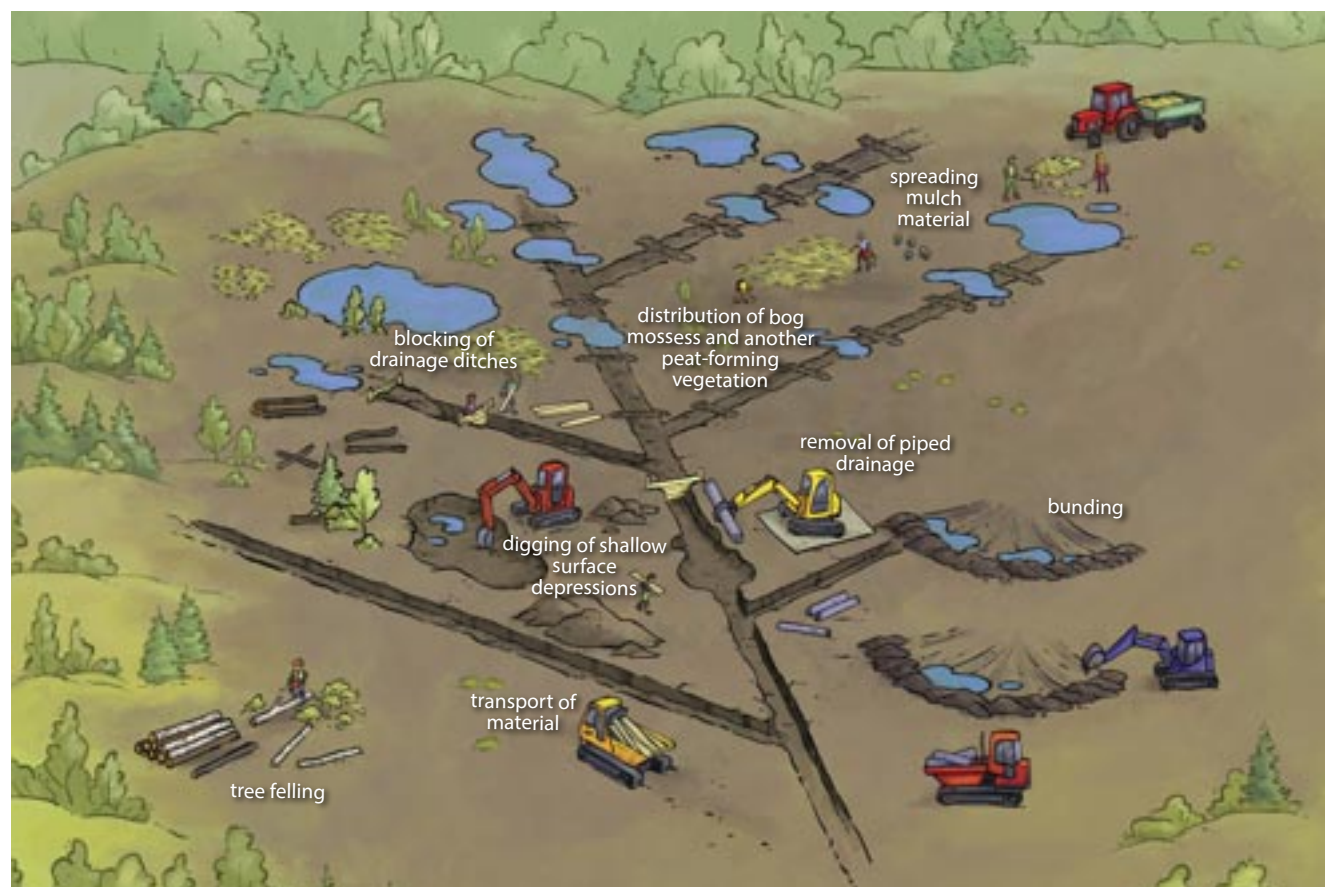
Fig. 90: Simplified drawing of various measures carried out during the restoration of an industrially mined peat bog
