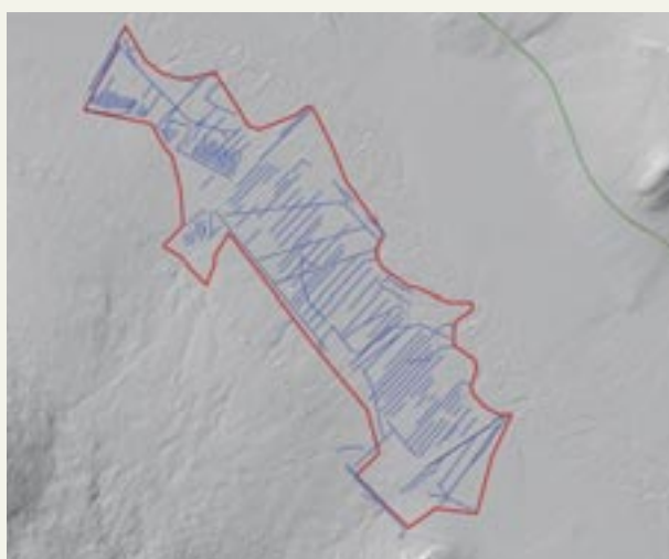
Fig. 231: Scheme of the drainage based on LIDAR images, Dobrovodské louky site
