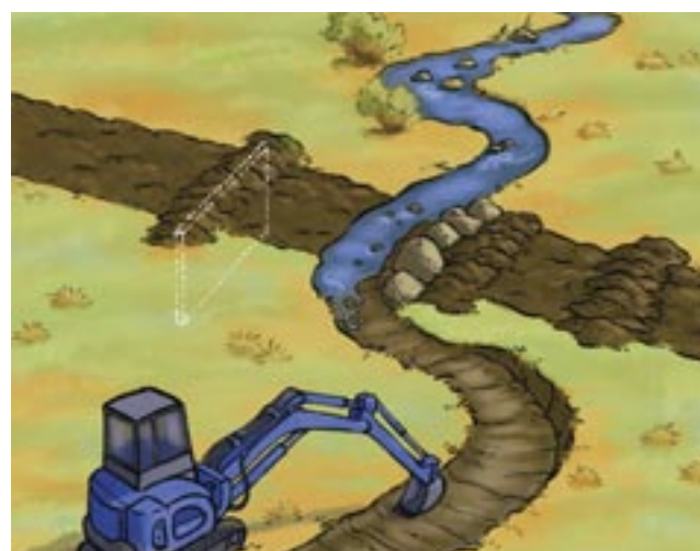
Fig. 129: A simplified drawing of the creation of a new stream cunette in the original route
