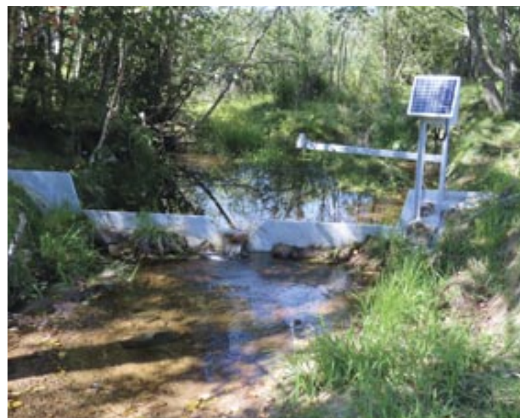
Fig. 192: Composite overflow and measurement set-up at the outflow from the Malý Bor site, September 2019 (T. Doležal)
