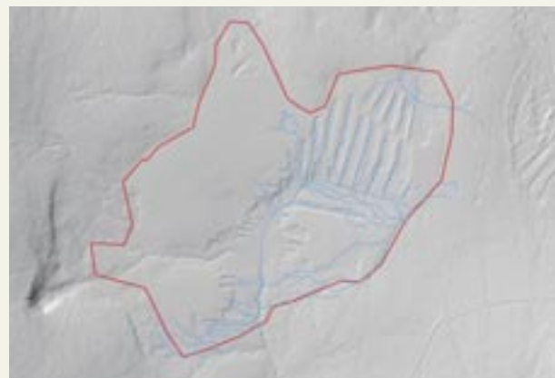
Fig. 253: Scheme of the drainage based on LIDAR images, Jezerní slat'
