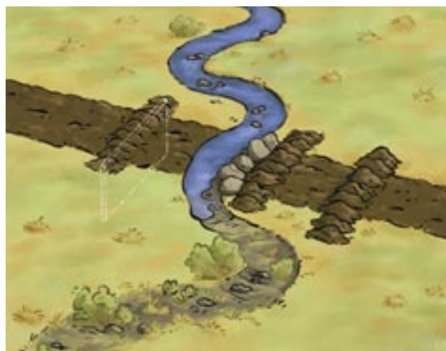
125: Simplified drawing of returning the stream to a preserved historical stream bed
