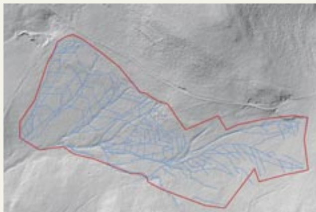
Fig. 237: Scheme of drainage based on LIDAR images, Rovina site
