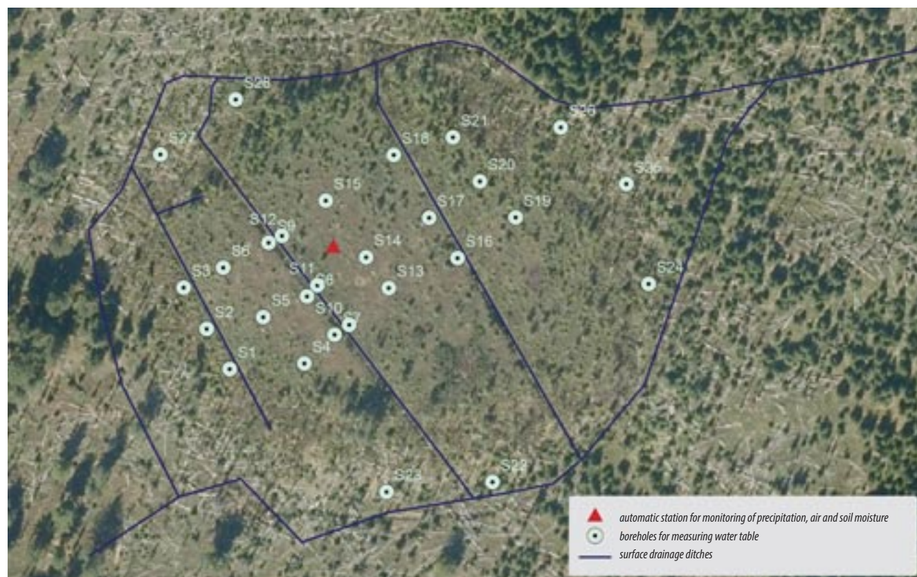
Figure 182: Design of the boreholes placement for measurements of water table on the restored Schachtenfilz peat bog.
