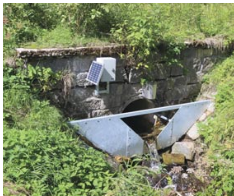
Fig. 191: Thomson spillway and measurement set-up at the final runoff from the Vchynice-Tetov site, September 2019 (T. Doležal)
