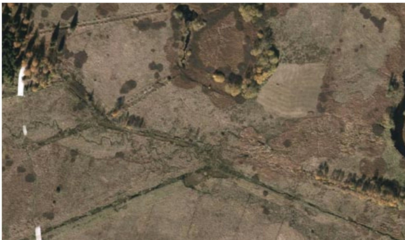
Fig. 133: The combination of the shaped cunette of the Žlebský stream with its returning to the preserved sections of the stream bed (on the left of the picture) and free release into the natural runoff route in the stands of tall sedges and reeds (on the right of the picture) on the background of an aerial photo. The start of the free releasing runoff is marked with a red dot.
