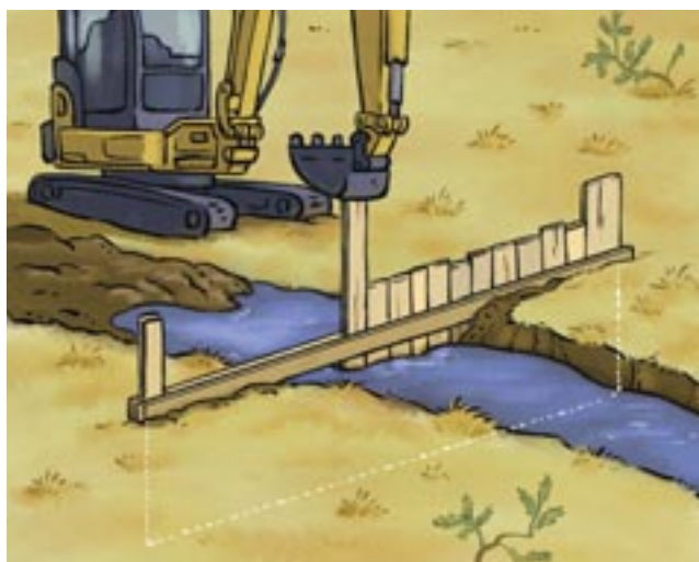
Fig. 63: Installation of a dam from vertical planks with help of technique
