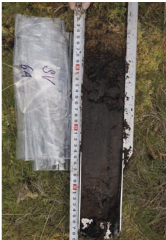
Fig. 199: Box corer with an intact peat sample.
