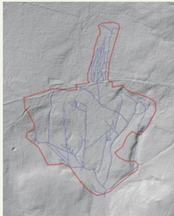
Fig. 212: Map of the hydrological situation and drainage based on LIDAR images
