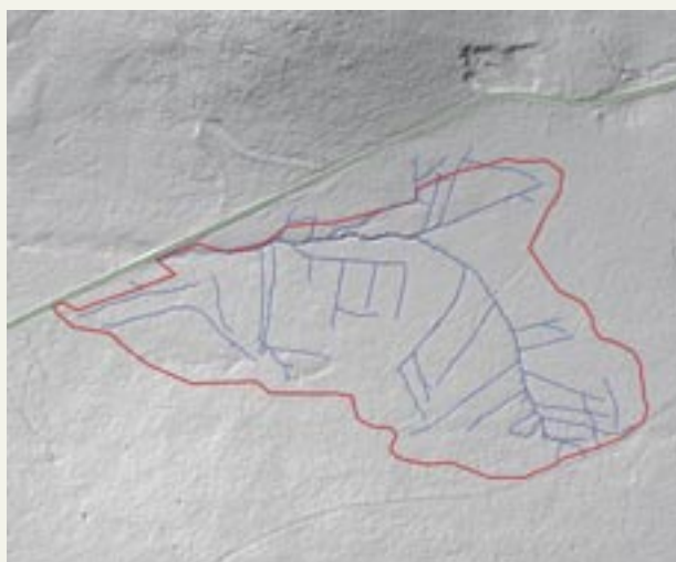
Fig. 226: Scheme of drainage based on LIDAR images, Gerlova Hut' site
