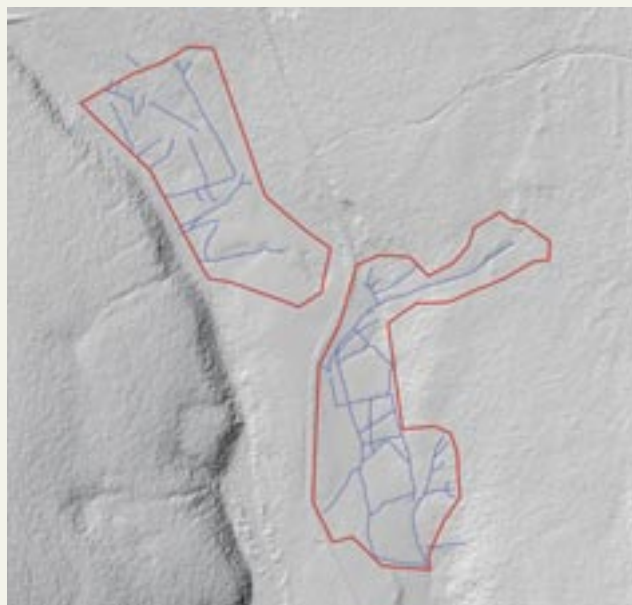
Fig. 222: Scheme of drainage system based on LIDAR images, U Tremľů site
