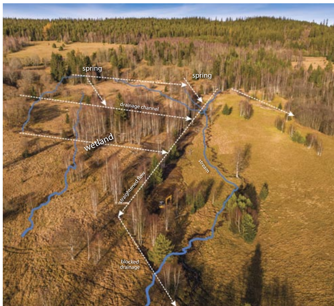
Fig. 45: An example of the hydrological restoration of a selected micro-catchment on the slopes in the Křemelná basin shows a joint solution of drained springs, wetlands and straightened water courses, location Pod Skelnou, 2022 (R. Plíhal).
