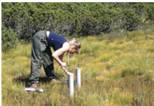
Fig. 181: Manual measurements of water table at the early beginning of mire monitoring in Šumava, Blatenská slat, August 2005 (P. Hájková)
