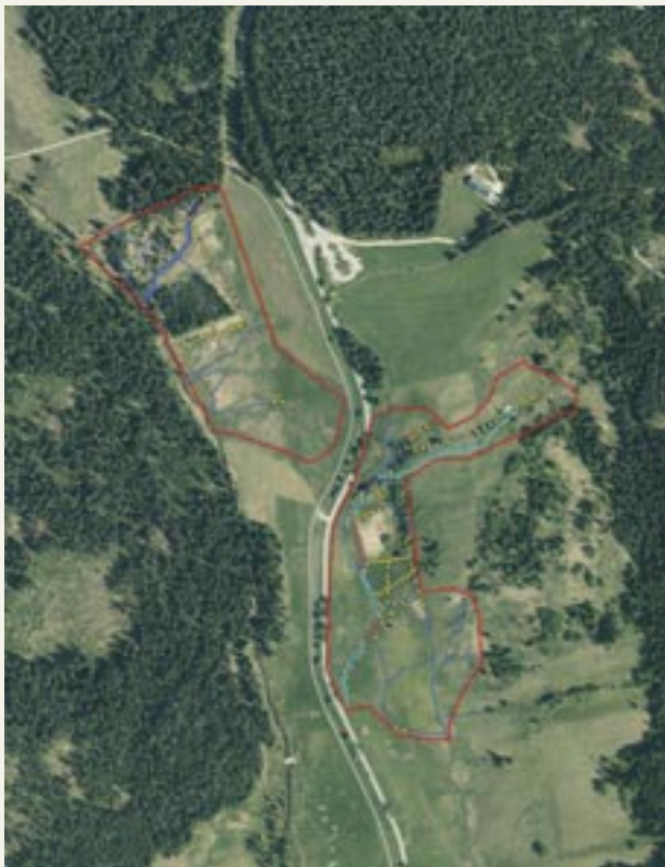
Fig. 224: The drainage scheme of the U Tremlů site and the measures taken on the basis of the aerial image. From the technical documentation (prepared by Geovision Ltd. 2021).
