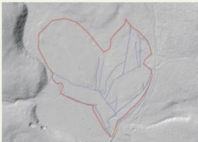
Fig. 207: Scheme of the Malý Bor site drainage based on LIDAR images
