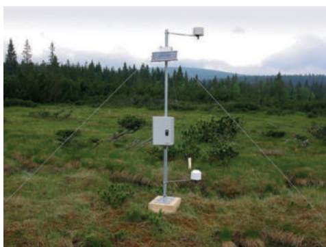
Fig. 3b. Microclimate station MC-SAR installed in BOG2 (Šárecká slat').
