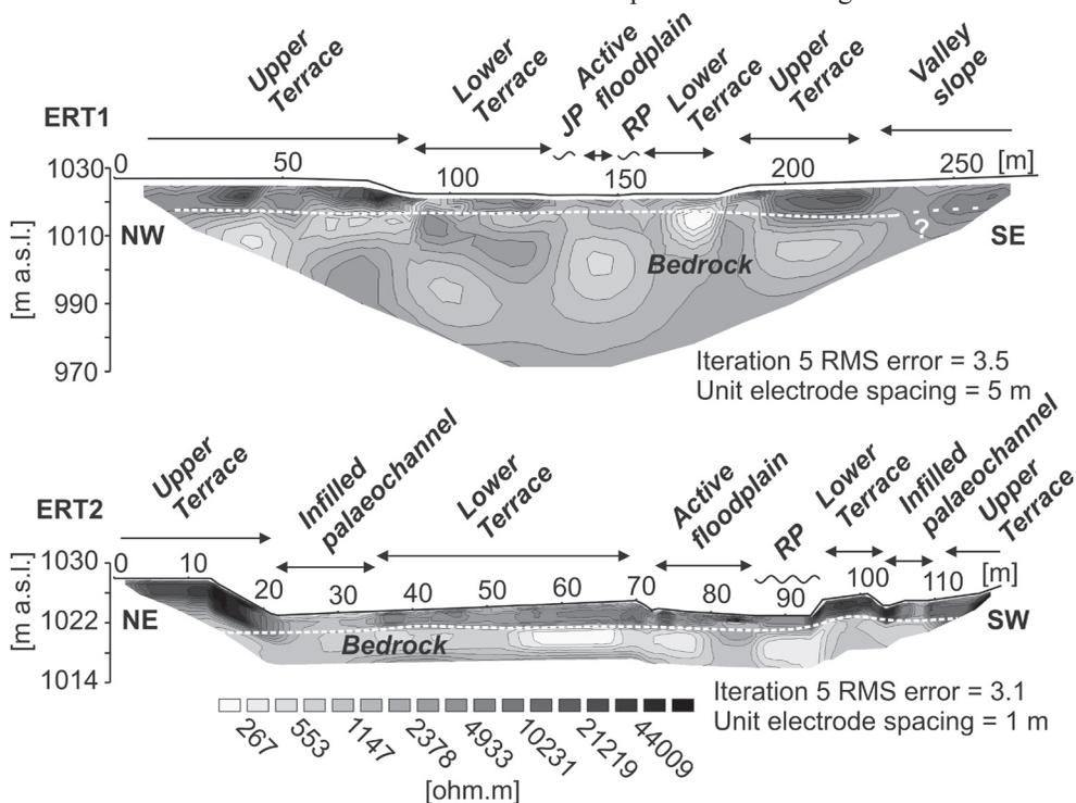
**Fig. 2.** Electrical resistivity profiles across the valley infill on the confluence of the Roklanský Potok and Javoří Potok streams. For the location of profiles, see Fig. 1. Sine curves indicate the location of the Roklanský Potok (RP) and Javoří Potok (JP) streams. Dashed line indicates the border between alluvial infill and the granitic bedrock.
