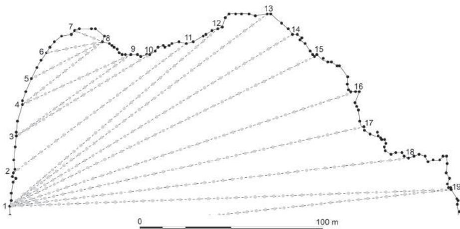
**Fig. 1.** Example of measured points at Čertovo Lake. Black points are points measured with the Leica total station on the lake shore (numbers represent the starting and ending points of depth profiles); the black line is at a distance of 5 m along the profile (dashed line).
