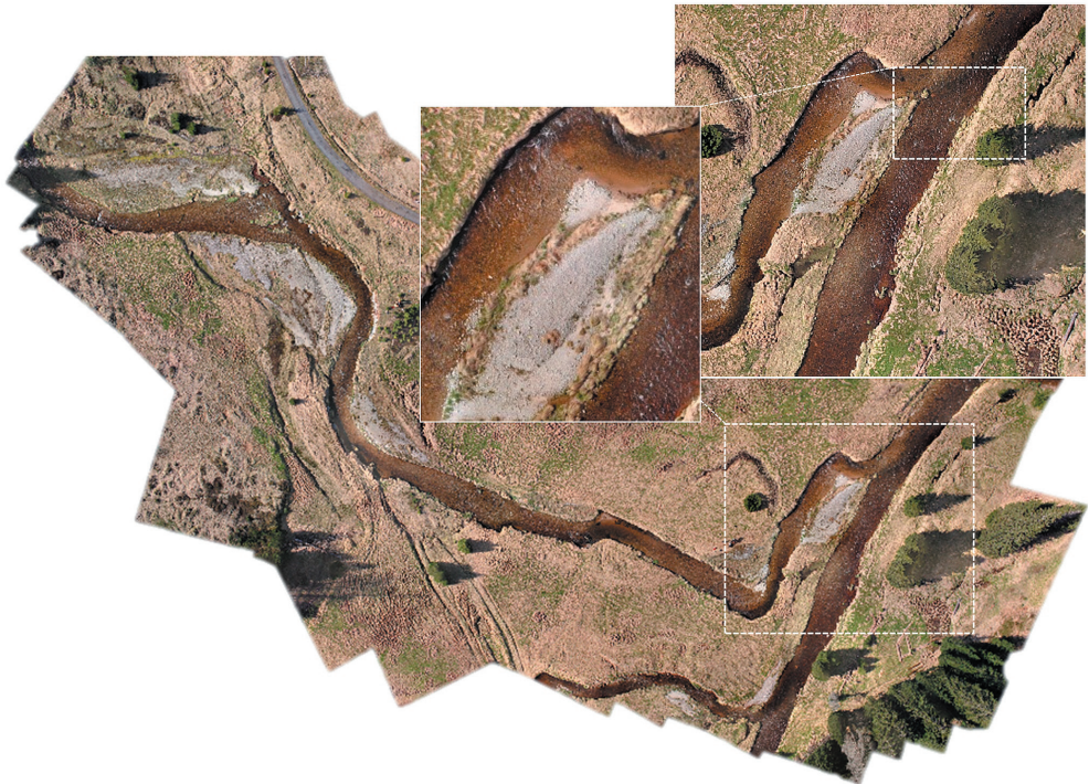
Fig. 4. The high precision digital elevation model (DEM), derived using UAS photogrammetry. The DEM resolution of 2 cm per pixel enables to perform highly accurate calculations of areal and volumetric changes in riverbeds and riparian zone.
