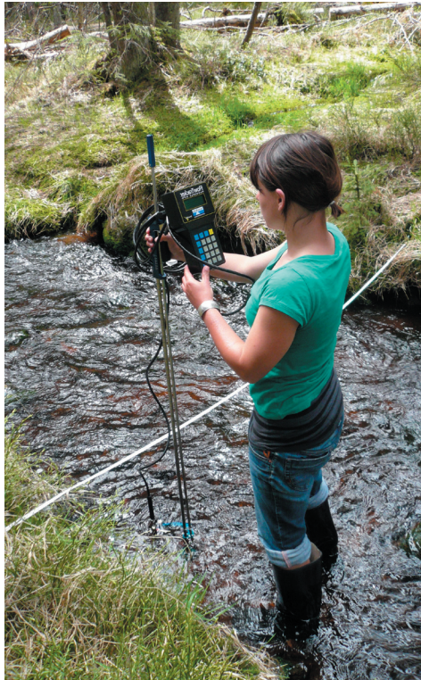
Fig. 2. Hydrological monitoring and survey: Automated sensor network, operated by the Charles University at the Březnický Potok gauging station (a); Hydrometric measurement using the FlowTracker velocimeter (b). Photo J. Langhammer, 2012
