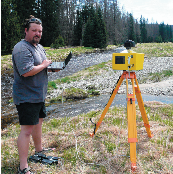
Fig. 3. The tools applied for research in fluvial geomorphology: The UAS platform MikroKopter Hexa XL applied for acquisition of detailed DEM (a); The terrestrial LiDAR scanning using Optech Illris 3D scanner (b). Photo J. Langhammer, 2013
