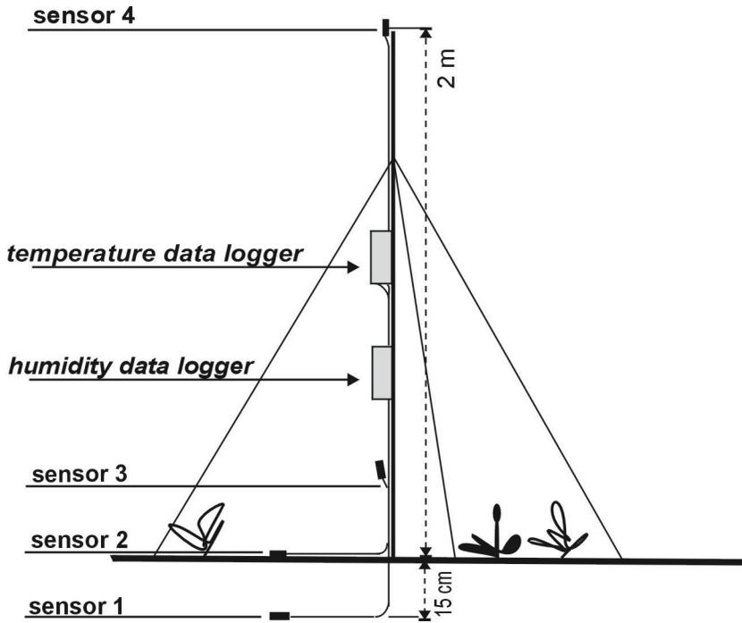
Fig. 2. Schematic picture of a data logger.
